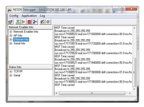
The Debug Window will show whether the unit is synchronised or not as well as other details about the units status. Clicking the 'Start Debug Log' button, allows the software to write the output information to a text file which can be saved and used to aid Technical Support Staff.
