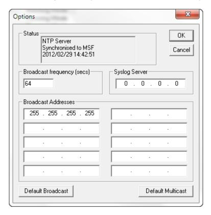
Broadcasts are a way of sending a single timestamp to many computers at the same time. Multicasts are similar but may span more than one subnet if the network is set to do so. If the value of the broadcast frequency is set to 0, none are sent.
